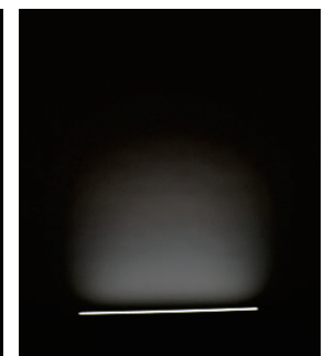
45° Front View Distance to the wall is 200mm[7.87in.] Graze height on the wall is 2200mm[86.6in.]
